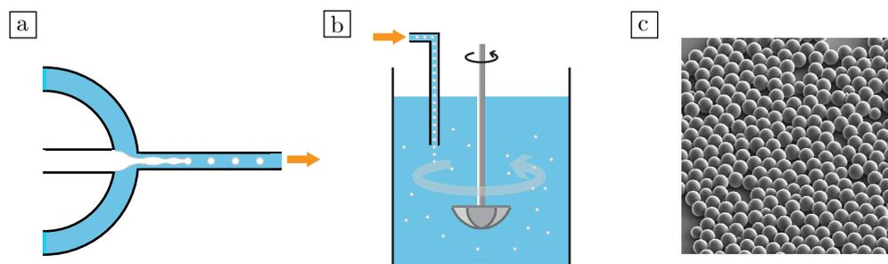
Figure 1: (a) Producing uncured droplets with a microfluidic chip. (b) Droplets are being stirred in a beaker to be cured into particles or capsules. (c) SEM image of nearly neutrally buoyant particles [1].
