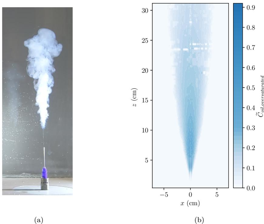
Figure 1: Converting recorded image in (a) to concentration field in (b)
