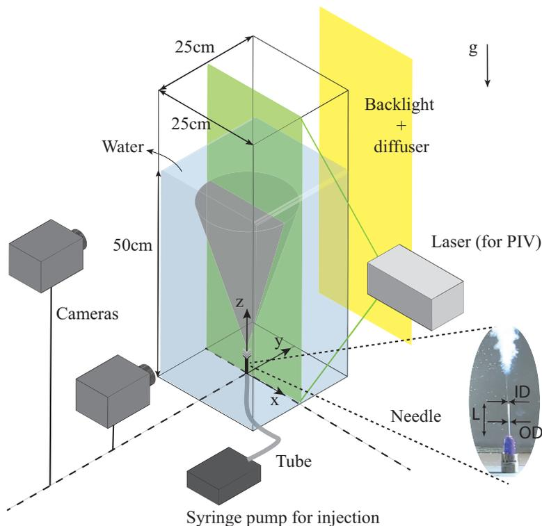
Figure 2: Experimental setup. The inset shows the photo of the needle for injection. Note that the laser was only activated for PIV.
