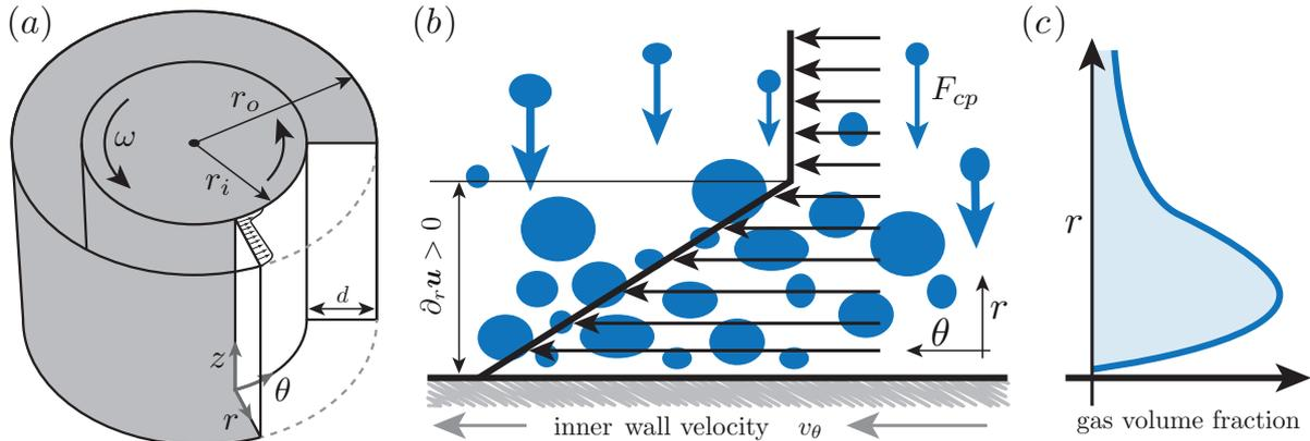
Figure 1: (a) Sketch of the Taylor–Couette flow. (b) Bubbles are pushed towards the inner cylinder into the boundary layer by the centripetal force. (c) A plot of the expected gas volume fraction as a function of radial distance — most of the bubbles are located in the boundary layer near the inner cylinder.
