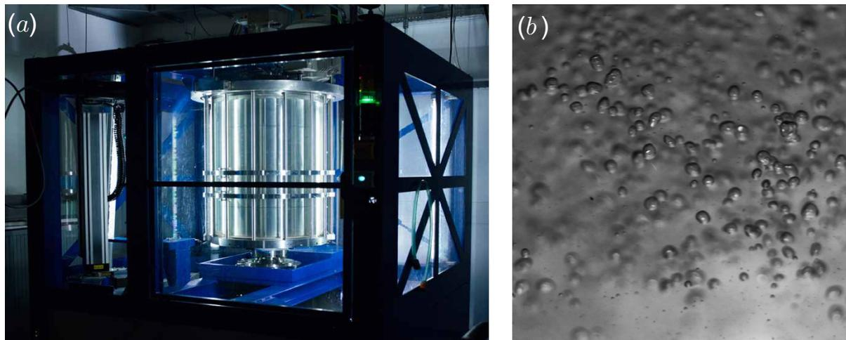
Figure 2: (a) Picture of the Twente Turbulent Taylor–Couette setup. (b) Snapshot of bubbles close to the outer cylinder.
