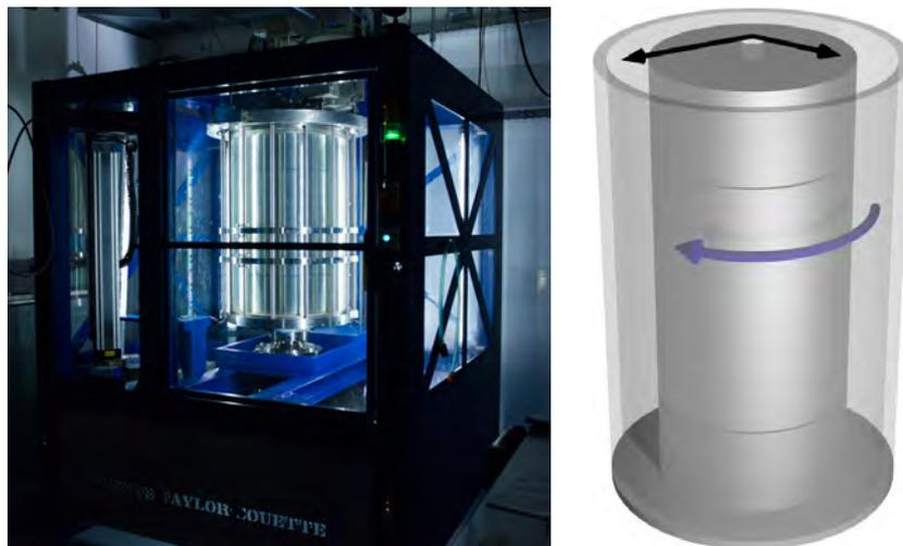
Figure 1: left: Photograph of the Twente Turbulent Taylor–Couette ( $T^3C$ ) facility. right: Artist's impression of the inner cylinder and transparent outer cylinder
