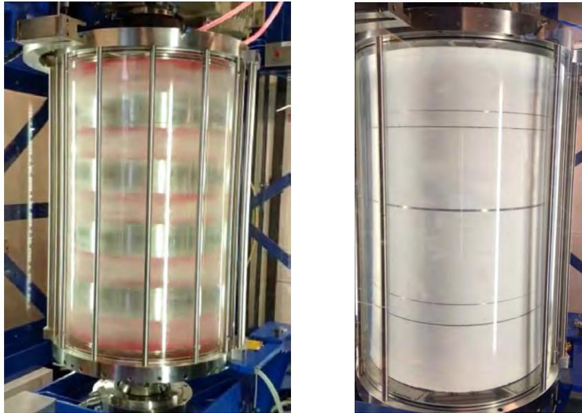
Figure 2: left: Still of a measurement in the Twente Turbulent Taylor–Couette ( $T^3C$ ) facility, with the inner cylinder covered with roughness patches (red bands). Air bubbles are introduced to the flow that are trapped in the regions of higher intensity turbulence, corresponding to the locations of the roughness patches. right: Photograph of the  $T^3C$  where the inner cylinder is covered by a superhydrophobic coating.
