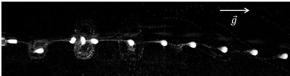
Figure 1 - Position of a cloud of particles in a vortical flow at different times
